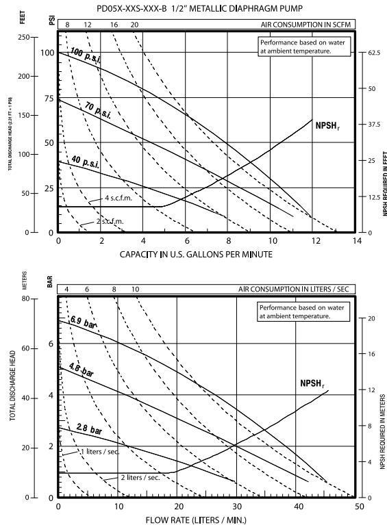
Performance based on an elastomeric fitted pump, flooded suction with water at ambient conditions. Due to varying materials of construction, assembly configurations and operating conditions, published data is for reference only
