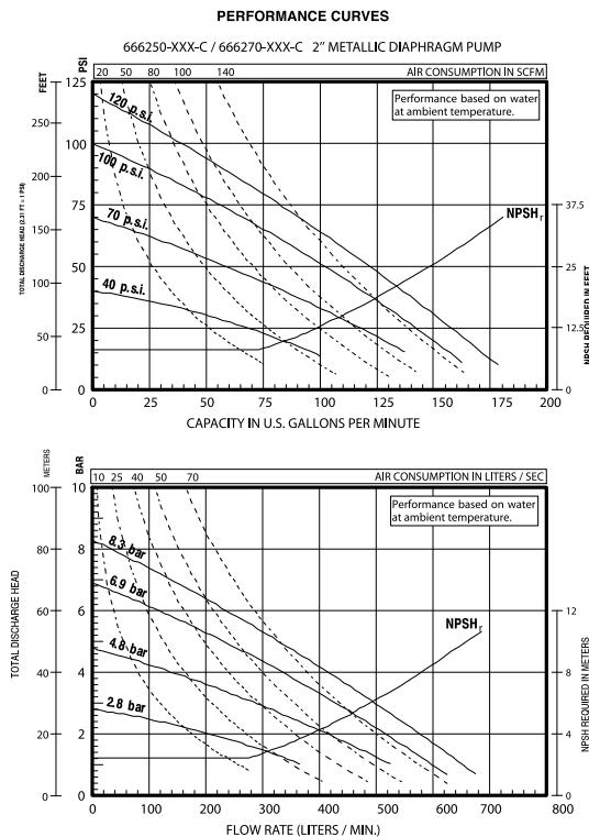
Performance based on an elastomeric fitted pump, flooded suction with water at ambient conditions. Due to varying materials of construction, assembly configurations and operating conditions, published data is for reference only.
